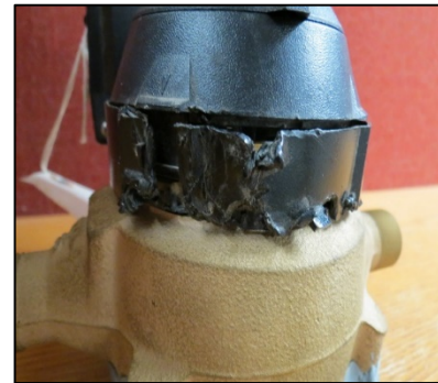
Tampered AMR meter reading device
