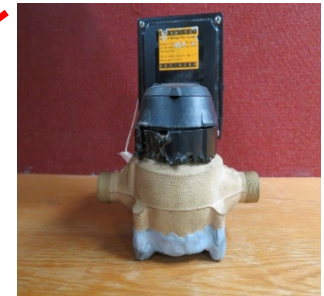
Tampered AMR meter reading device
